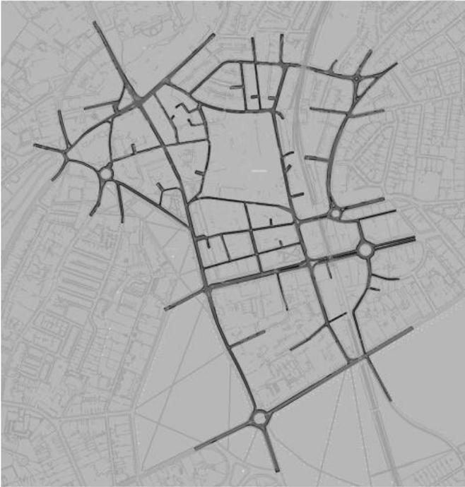
A programme of traffic survey data collection was undertaken in July 2018 and used along with other available data to form an understanding of traffic patterns and network conditions. The survey data, along with traffic signal information and bus service data was used to develop the 2018 base model.
