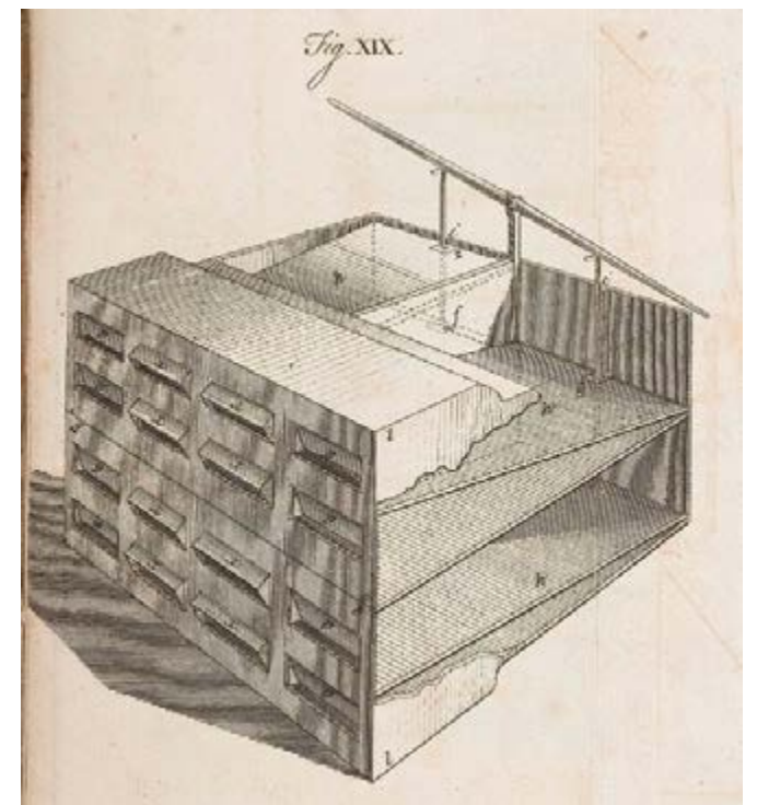
Ventilation bellows designed by Dr Stephen Hales
