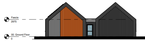
South Elevation Block A 1 : 100
