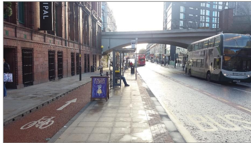
Figure 3.9. Segregated cycleway (carriageway height)
